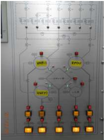
Schematic diagram of PECVD with Load-lock and gas flow system
