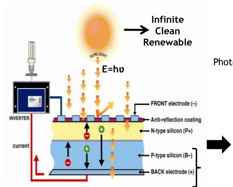
Basic Principle of Solar Cell Operation
