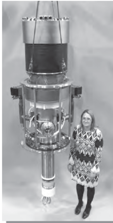
Monica Blank, Chair of VETC, standing next to a 170 GHz, 1 MW power level gyrotron oscillator
